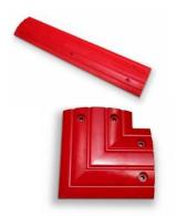
Made from Heavy Duty UV Stable Urethane, DuraBund is especially designed to withstand the rigors of workshop traffic. It will easily withstand car, forklift and heavy truck access. Excellent chemical resistance makes it ideal for bunding most class 8 corrosives, class 5 oxidisers and other non-flammable liquids. Pre-formed anchor points for dynabolts and right-angle corner pieces mean you can simply install DuraBund to suit any size configuration.
