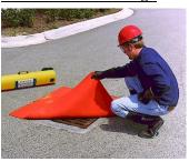
The Ultra-Drain Seal provide overlap on most New Zealand drains. The reinforced mesh is 'sandwiched' between different layers of polyurethane and increases durability and resistance to tearing. This could be a valuable addition to any emergency response plan, spill kit or Stormwater management program. It resists oil, water and most aggressive chemicals and cleans with soap and water.
