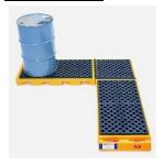
The Ultra-Spill Deck is a polyethylene construction and offers a wide range of chemical compatibility. Its low profile design offers safe and convenient loading and unloading of drums without the need for a hoist. The drum has a weight of 10kgs and a uniformly distributed load of 681kg. The containment capacity is 42 litres. The Ultra-Spill Decks are available in 1,2 and 4-drum modules.
