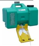
The Gravity Fed Eyewash is made from UV stabilised high density polyethylene the portable 35 litres gravity fed eyewash unit provides a minimum of 15 minutes of continuous flow. The spray nozzles are protected from dust, grime and damage when the tray is in closed position. The wide fill opening with threaded cap permits easy inspection, cleaning and filling.
